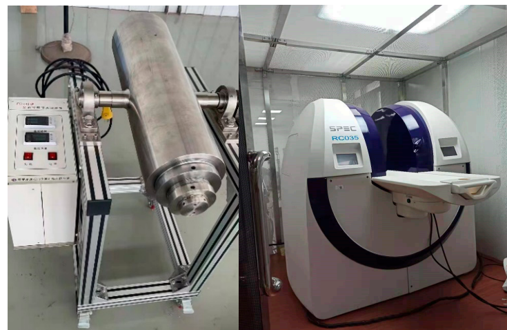
Figure 2. Full-diameter core holder (upper left) and Spec-RC035 large NMR scanner (upper right).
