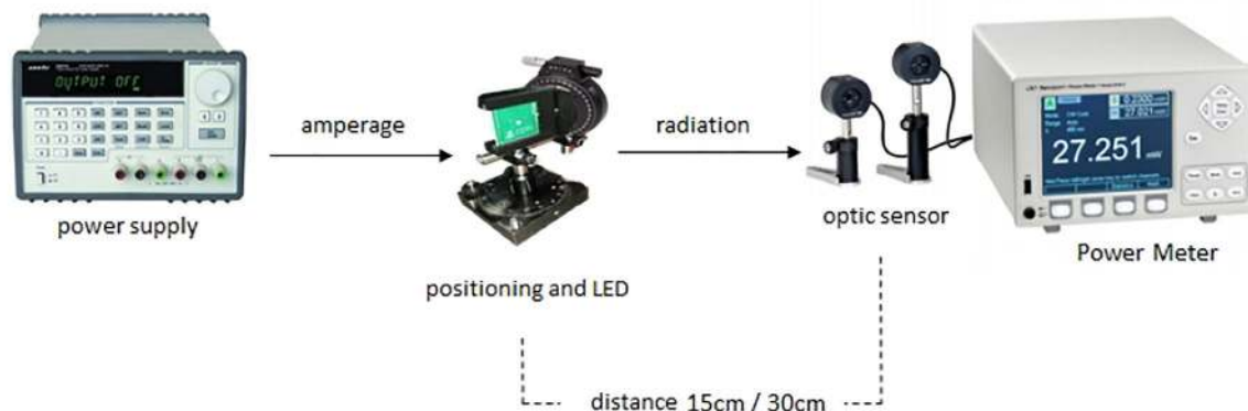
Figure 4. Schematic diagram made for measuring LED power
