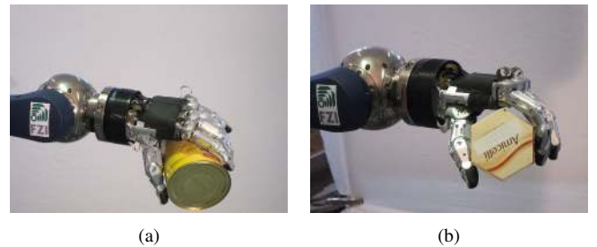
Fig. 7. Grasping of large objects. The tin in Fig. (a) has a diameter of 10 cm. The grasp for this object cannot provide form closure.
