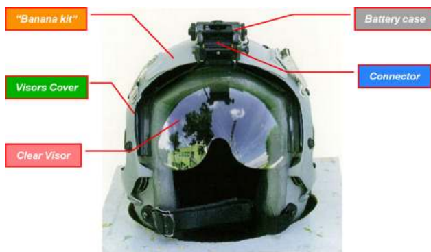
FIG. 7 Modified HGU-55/G helmet with NVGs installed.
