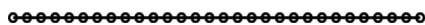
Fig. 2 Schematic representation of the finite element mesh of the free-free beam shown in Fig. 1
