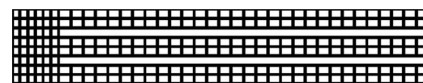
Fig. 10 Schematic representation of the finite element mesh of the clamped plate with slots shown in Fig. 6
