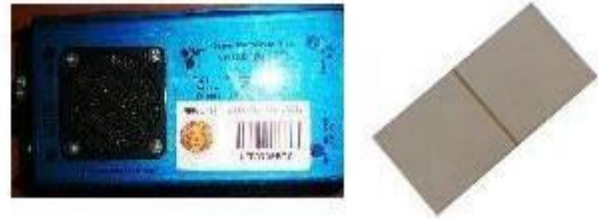
Fig.4 Bimorph piezoelectric actuator with amplifier
