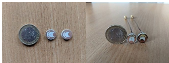
Fig. 2. Fabricated in-body antennas (a) antennas without coaxial cable. (b) antennas with coaxial cable.
