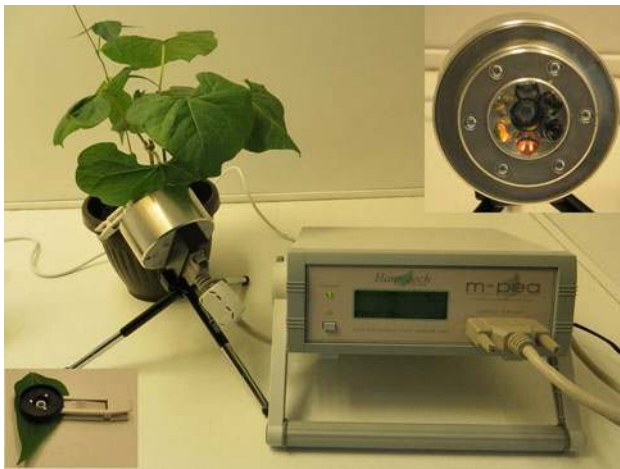
Fig. 8 M-PEA (of Hansatech company, UK). It allows one to measure several signals: PF (Chl a ), DF (Chl a ), P700 absorbance change, and relative chlorophyll content. The device electronically separates the signals of prompt and DF using fast switching light-emitting diodes as the light sources, and sensitive photodiodes as the light sensors. The light emitters and sensors are placed in an optical sensor unit (shown as inset on the top right corner ). The optical sensor unit is fixed on a tripod and has 3D mobility, making it convenient to use different plant samples. On the sample holder (leaf clip, see inset on bottom left corner ), leaf is fixed to the optical sensor unit; further, the sample holder protects the leaf and the sensors from extraneous light. The figure also shows a 30-day-old decapitated bean plant (ready to be used for an experiment; see Yordanov et al. 2008). Photograph by one of the authors (VG)
