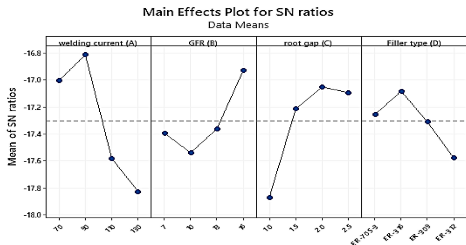
Figure 22. Main effect plot for S/N ratios of Bead Widths.
