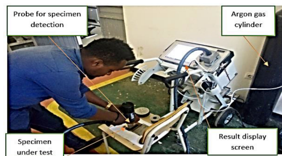
Figure 1. Setup ARC-MET8000 spectrometer (Ethiopian Technical University).
