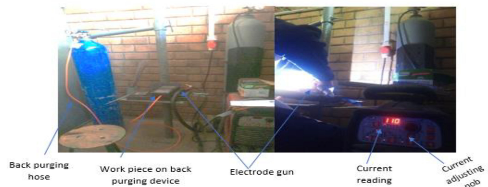
Figure 4. GTAW welding setup (Centre of Excellence for Engineering, Addis Ababa, Ethiopia).
