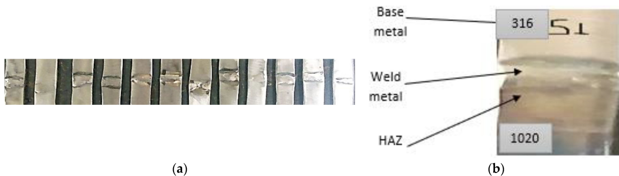
Figure 10. (a) Specimen prepared for hardness test; (b) three zones of samples.
