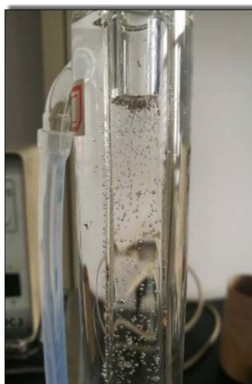
Figure 5. Apparatus setup for sand suspension ability test.
