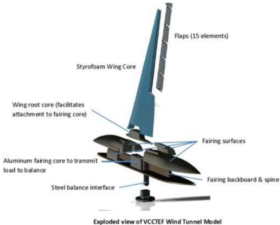
Fig. 13 - Exploded View of Wind Tunnel Model (Courtesy of University of Washington Aeronautical Laboratory)
