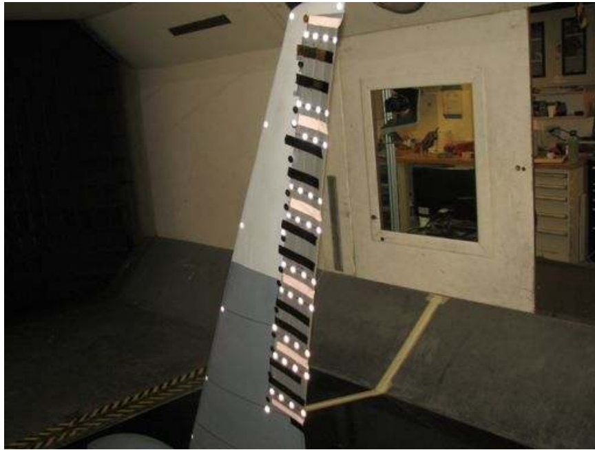
Fig. 61 - Wind Tunnel Model with VICON Dots in UWAL Test Section (Courtesy of University of Washington)
