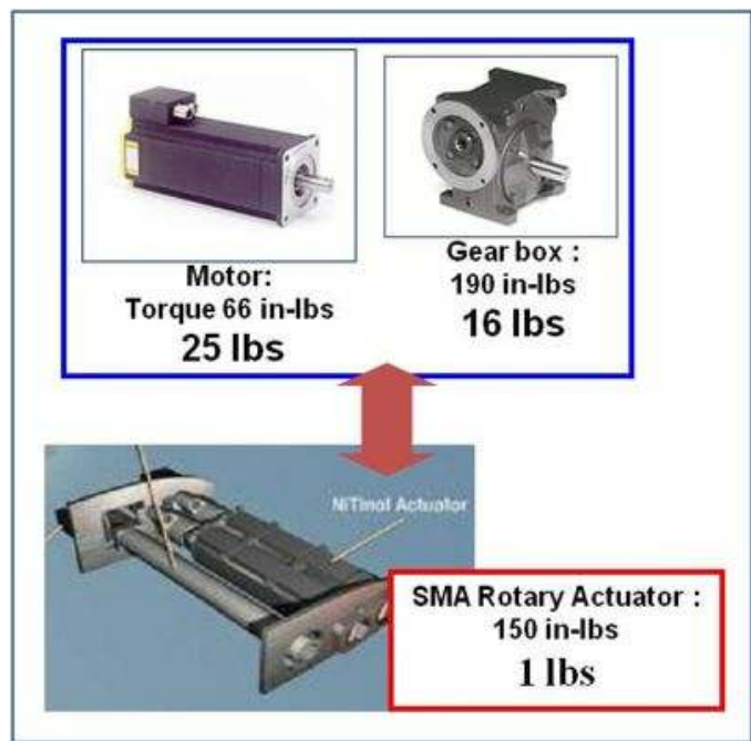
Fig. 4 - Shape Memory Alloy Actuators Have a Low Weight Compared to Electric Motor Actuators
