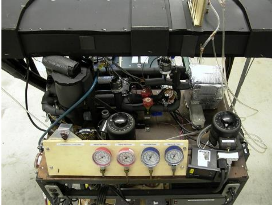
Fig. 2: Photograph of bread board miniature-scale refrigeration system for electronics cooling.
