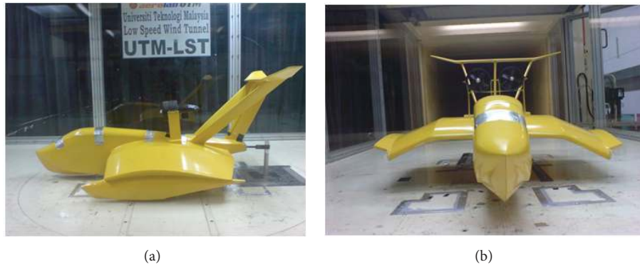
FIGURE 4: Wind tunnel test for WIG craft model: (a) model with endplates and (b) model without endplates.
