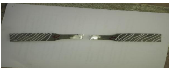
Fig. 3 Fractured tensile specimen
