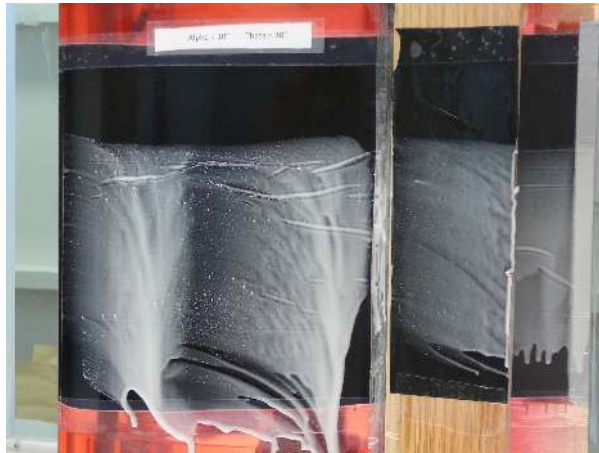
Figure 4.4: Oil flow on the fixed-deployment-angle effector at \theta = 30^\circ and \alpha = 10^\circ . Flow is attached on the effector as seen by the downstream movement of the oil.
