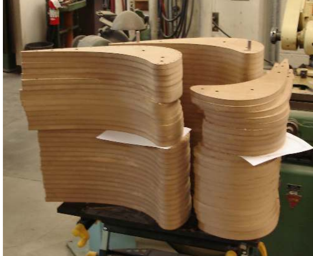
Figure 17. Rotor Blades During Construction
