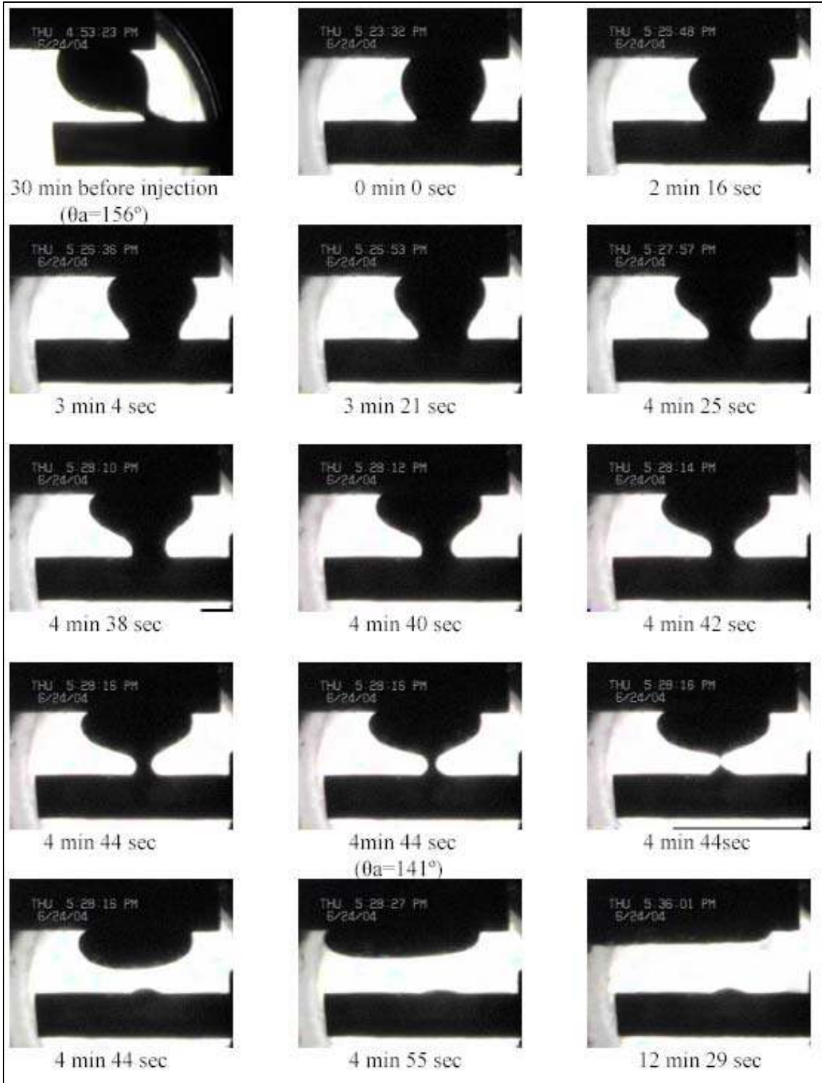
Figure 37: Depiction of Drop Movement During Surfactant Injection (Anionic Surfactant B at 3500 ppm, 700 psi and 82 °F, Yates stocktank oil)
