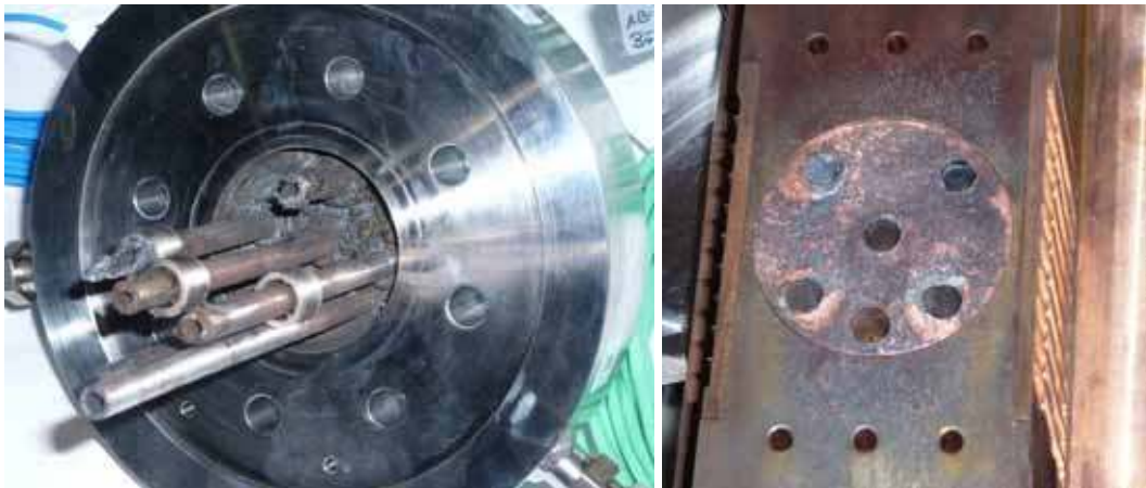
Burned LOx posts
