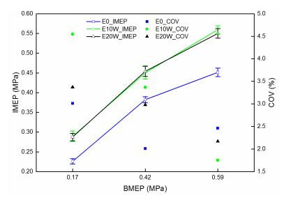
Figure 6. The cycle-by-cycle variations in IMEP for E0, E10W and E20W under three various loads.
