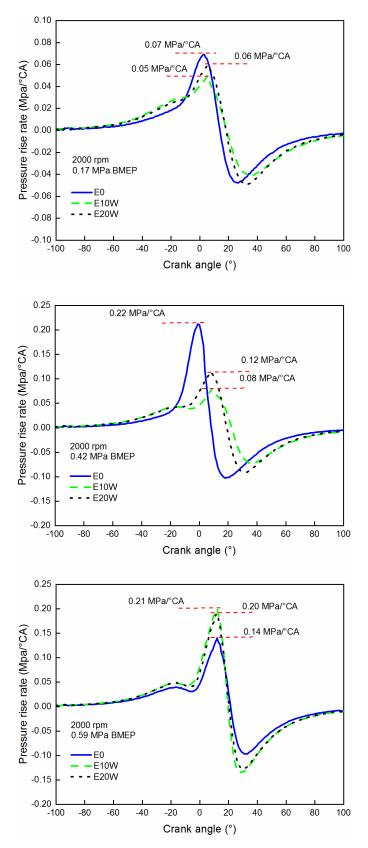
Figure 5. The average pressure rise rate of E0, E10W and E20W for three various loads.
