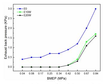
Figure 3. Exhaust back pressure of three fuels at various loads.
