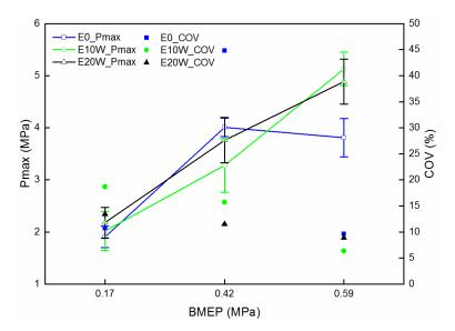
Figure 8. The cycle-by-cycle variations in *Pmax* for E0, E10W and E20W under three various loads.
