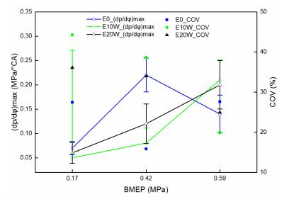
**Figure 7.** The cycle-by-cycle variations in  $(dp/d\varphi)_{max}$  for E0, E10W and E20W under three various loads.
