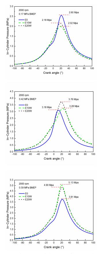
Figure 4. The average in-cylinder pressure of E0, E10W and E20W for three various loads.
