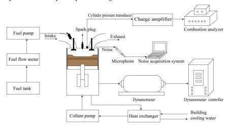
Figure 1. The schematic diagram of the experimental bench.
