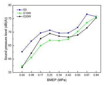
Figure 2. Noise emissions of three fuels at various loads.
