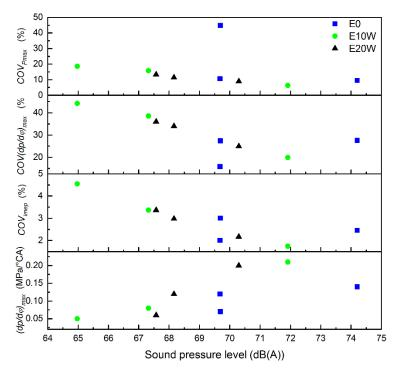
Figure 9. The relationship between noise emission level and combustion parameters.
