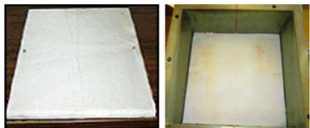
Fig. 2 Modification to the direct shear box
