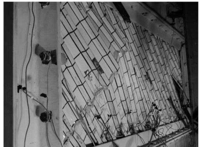
Fig. 11. Global and local buckling of Specimen C1 at -3\Delta_y of Cycle 16
