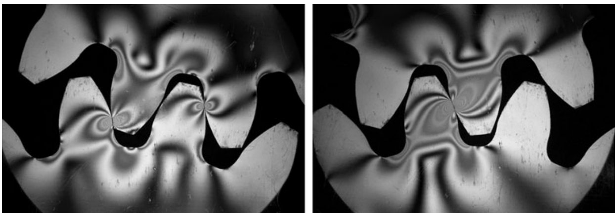
Figure 5: Isochromatic fringe patterns obtained by photoelasticity for double tooth contact (left) and single tooth contact (right)
