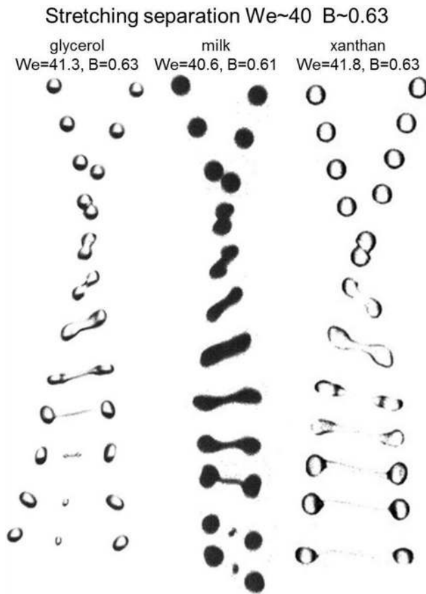
Fig. 8 Collision of 40 v% glycerol, 20% TS milk, and 500 ppm xanthan droplet collisions at We \sim 40 and B \sim 0.63
