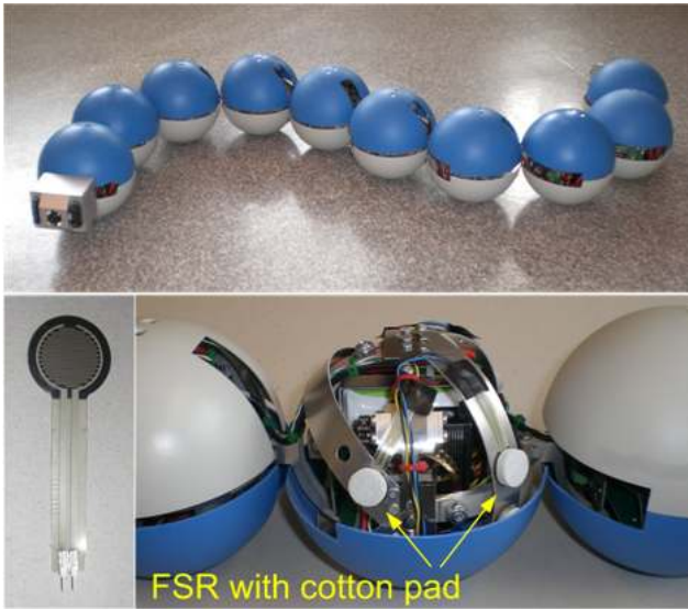
Fig. 4. Top: The snake robot used in the experiment. Bottom: The contact force sensor system of the robot.
