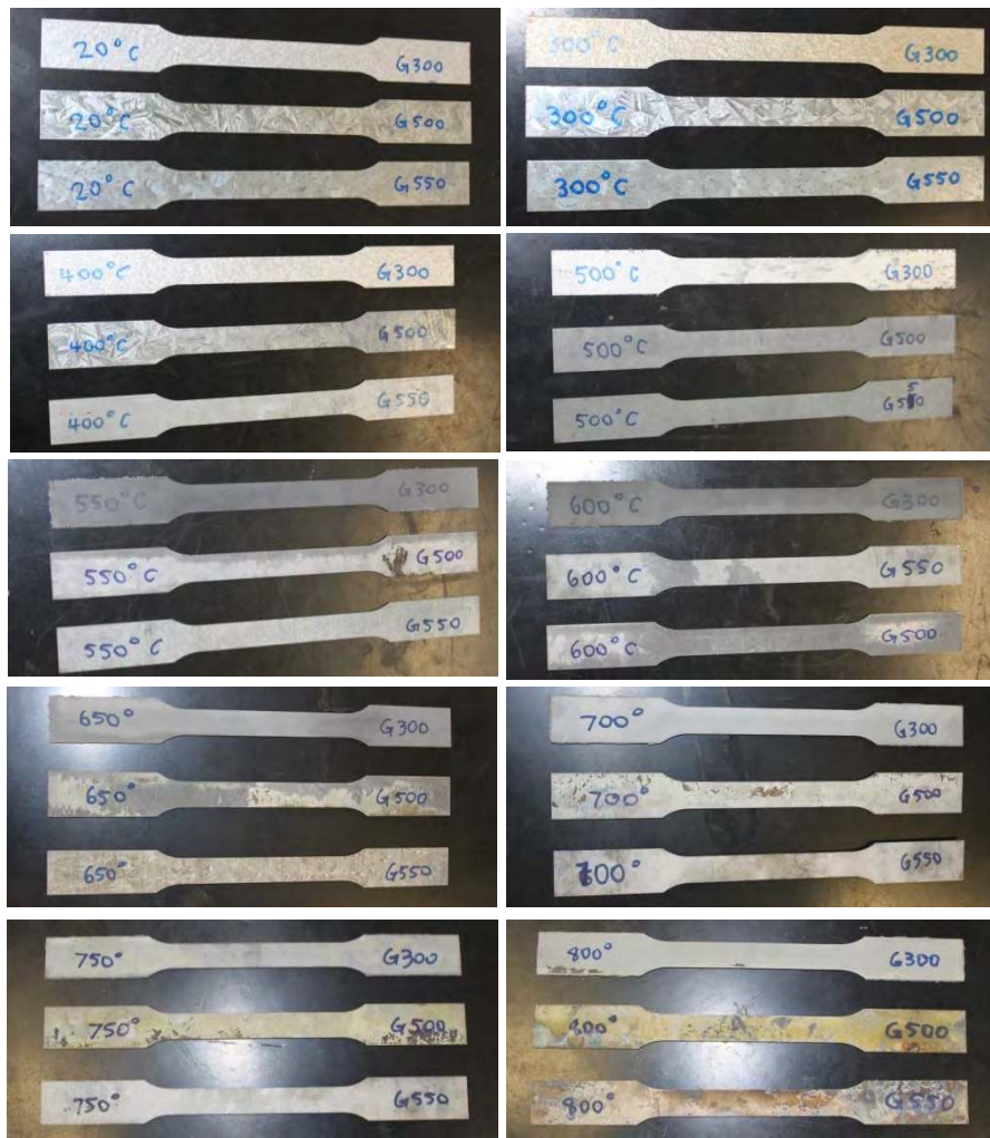
Figure 6: Test specimens after being exposed to elevated temperatures
