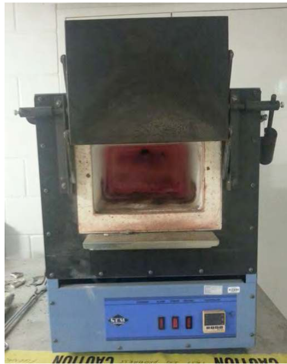
Figure 4: Electric furnace used for heating the test specimens
