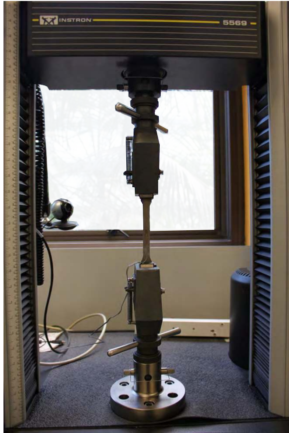
Figure 5: Tensile test set-up
