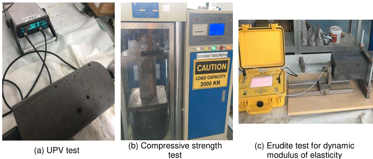
Fig. 4. Tests facilities for concrete cylinders and prisms
