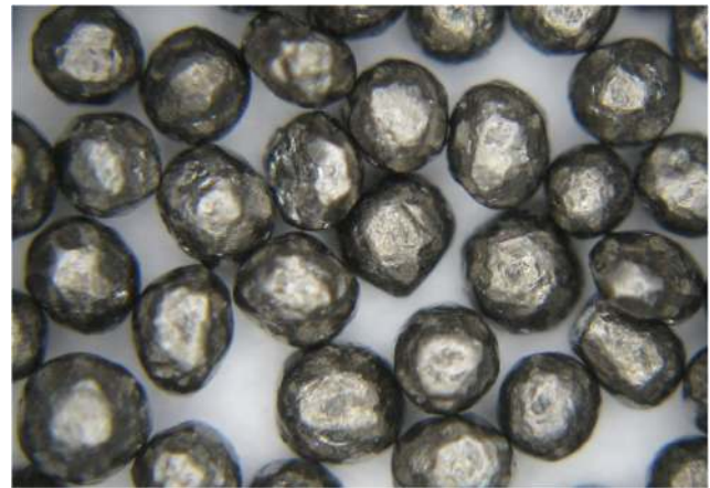
Fig. 4 Cut wire shot peening media with nominal diameter 0.7 mm. This media had been used in the shot peening machine for a long time
