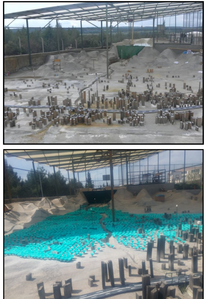
Fig. 1. Physical model of Urkmez Dam Lake and downstream region without vegetation and with vegetation.
