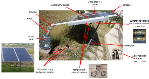
Figure 3. Experimental setup and designed cooling system.
