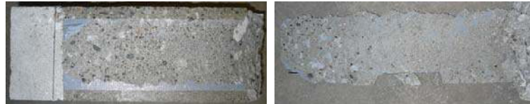
b. failure within concrete substrate (B-3 series)
