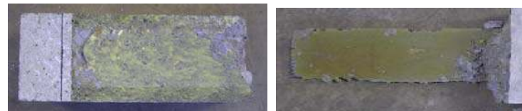
e. failure at primer to concrete interface (B-7 series)
