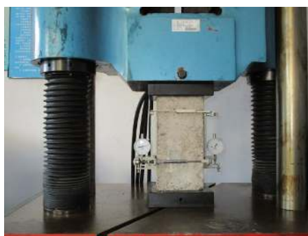
Figure 5. Modulus of elasticity test.
