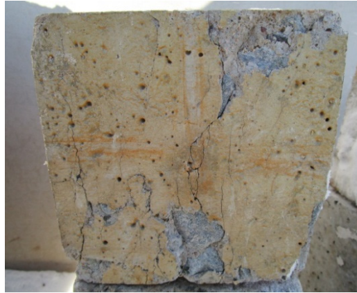
Figure 7. Sulfate corrosion for crumb rubber concrete.
