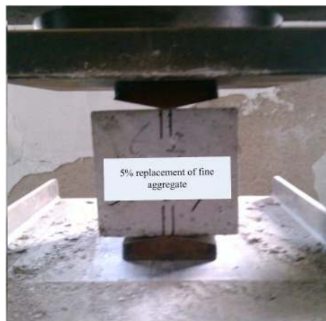
Figure 4. Splitting tensile strength test.
