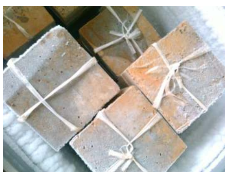
Figure 6. Freezing-thawing of crumb rubber concrete.
