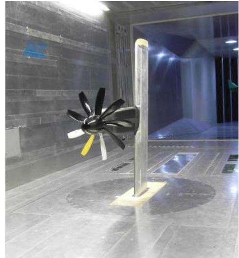
Figure 5. experimental setup in test section of DNW-NWB.
