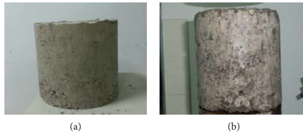
FIGURE 22: Appearance of test specimen (a) before and (b) after the freeze-thaw cycle. (a) Standard curing specimen. (b) Specimen after the fifth freeze-thaw cycle.
