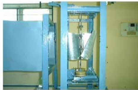
Fig. 5. Twisted bladed rotor at the tunnel exit
