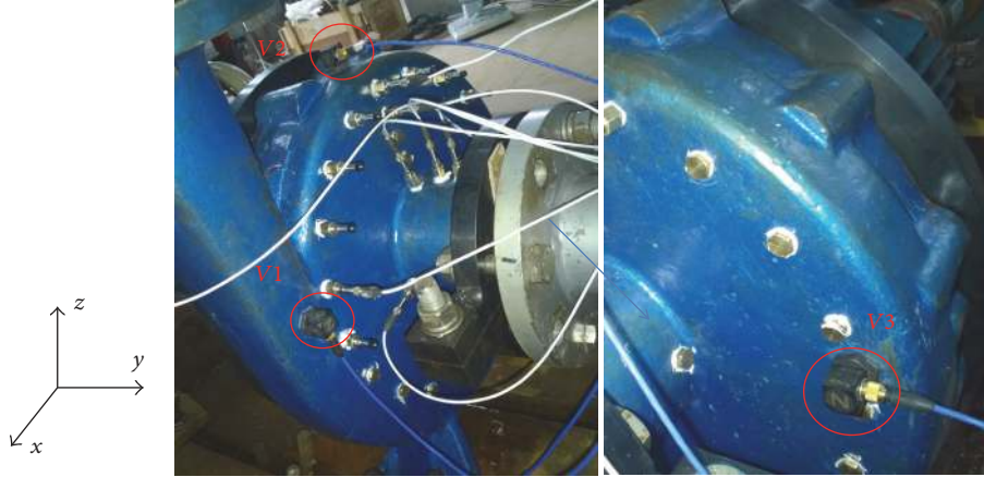
FIGURE 2: Positions of the accelerometers mounted on the volute casing.
