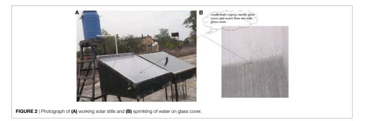
flow water at ambient temperature over the glass surface from period of 0800 to 1600 hours with the flow rate of 0.0001 kg/s. The flow rate was optimized by Somwanshi and Tiwari (2014). The depth of saline water is kept constant at 5 cm for the all sets of experiments.
