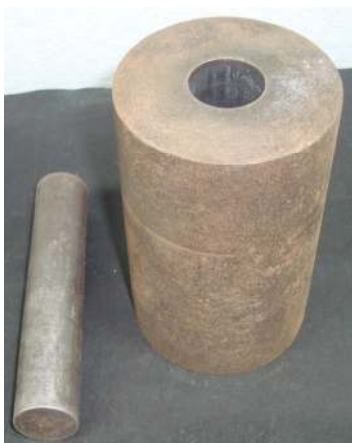
Figure 4. Metallic die with punch.
