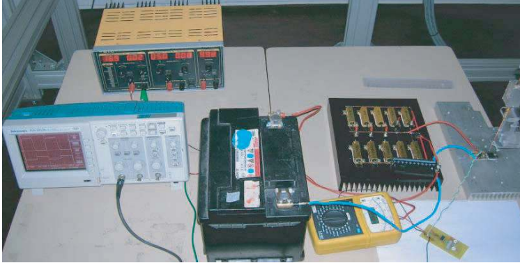
Figure 1. Experimental setup considered for the test of MOSFET.
