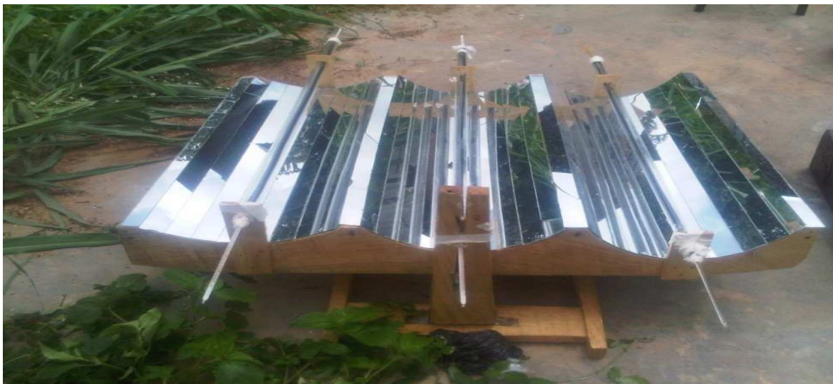
Fig. 1: Prototype line focus concentrating collector
