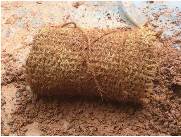
Fig. 2 Photograph of sample prepared for soil burial study
