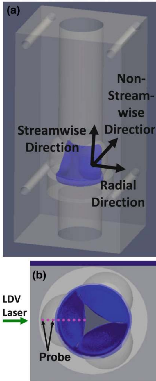
Fig. 3. (a) Definition of directions of velocity and shear stress measurements. The streamwise direction is defined as the direction pointing downstream, while the non-streamwise direction is defined as the direction from one commissure to the next. (b) Schematic of LDV velocity measurement scheme. Velocities were measured at intervals of 89 microns along a straight line at the center of the valve leaflet
