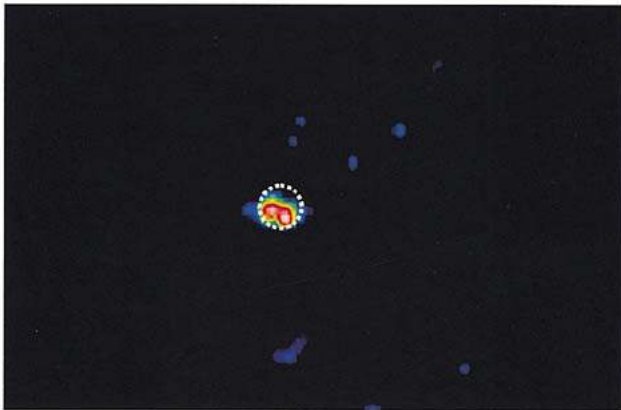
Fig. 13. Image formed of TS-50 AP mine (outlined) and clutter below pine straw surface cover in an 80\text{ cm} \times 120\text{ cm} scan region on a 25 dB scale.
