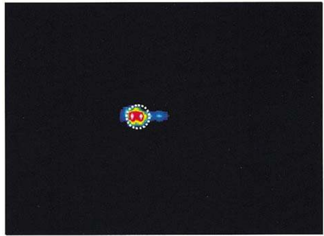
Fig. 9. Image formed of a single TS-50 AP mine (outlined) buried 1.3 cm deep in an 80 \text{ cm} \times 120 \text{ cm} scan region on a 25 dB scale.
