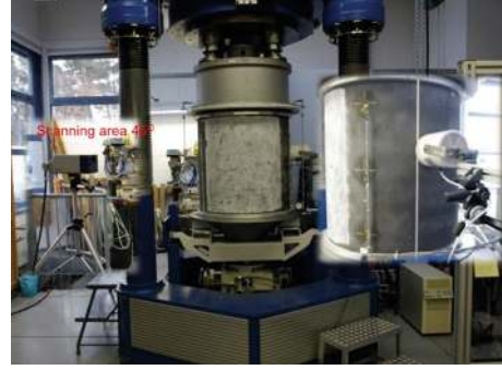
FIGURE 6: Experimental test setup for compressive loading on Z37 cylindrical shell (DLR).
