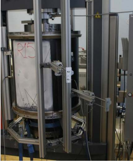
FIGURE 4: Experimental test setup for compressive loading on R15 and SST-1 cylindrical shells (RTU).
