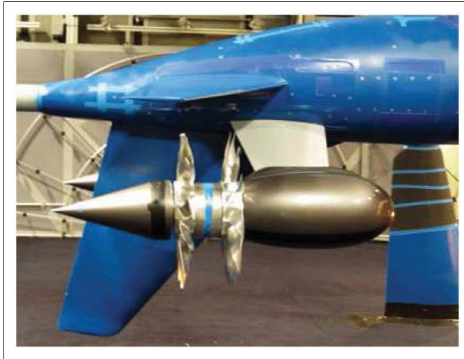
Figure 3. Installed CROR engine in pusher configuration.
