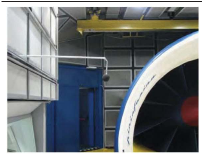
Figure 2. Out-of-flow microphone used for background measurements.
