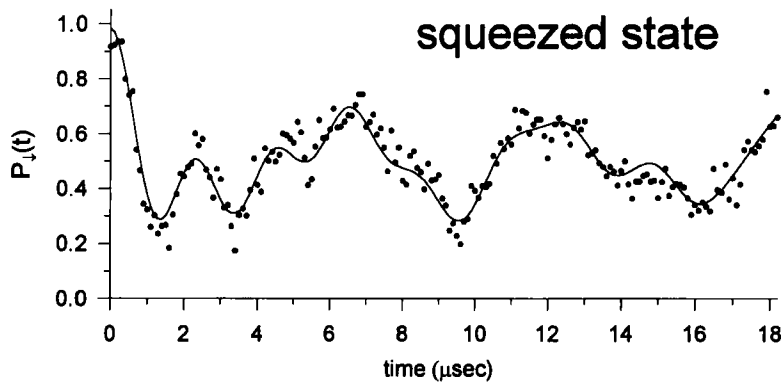
Figure 6. P_1(t) for a squeezed state. The data are fitted to a squeezed state population distribution, yielding \beta \approx 40 \pm 10 (16 dB below the zero point variance), which corresponds to \bar{n} \approx 7.1 .
