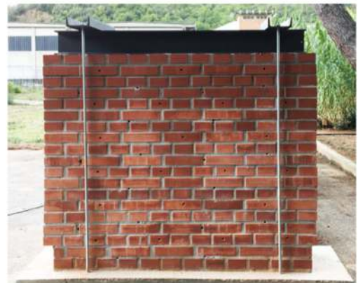
Fig. 3 Contrast system for the application of pre-stress on wall A through 2 + 2 steel bars—units in cm
