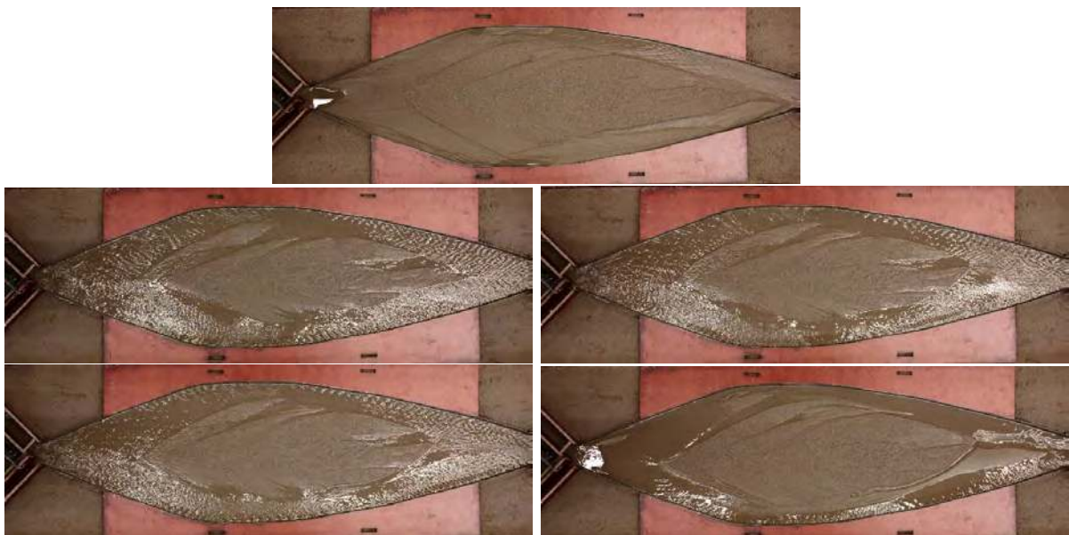
Figure B.9: Photo's taken at distinctive moments during the experiment. Starting up top: formation island. The low flow stage at t=15 min, at t=45 min, at t=75 min, at t=75 min empty.
