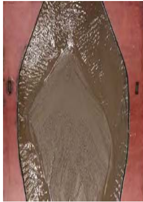
Figure 3.3: The asymmetrical formation of the bar/island due to the asymmetrical tributaries of the upstream confluence.
