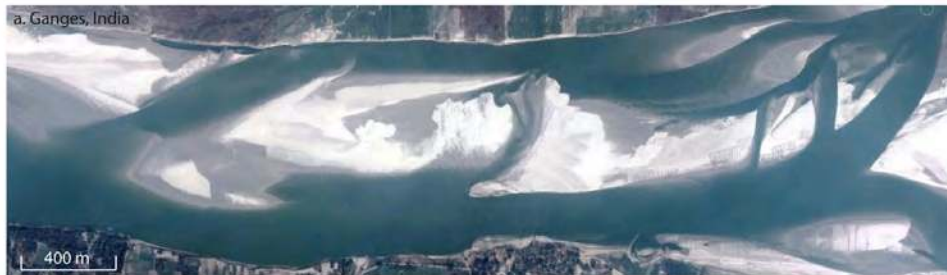
Figure 2.6: Formation of cross-bar channels in the Ganges River. Flow is from left to right, from (Schuurman and Kleinhans, 2015).
