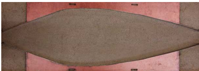
Figure A.7: The widened section with the wooden molds and stainless steel outer banks.
