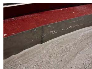
Figure A.7: The widened section with the wooden molds and stainless steel outer banks.
