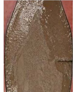
Figure 5.2: Direct bypassing of the weir.
