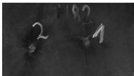
Fig. 17. Details of first and second shots hit damage on State A plate
