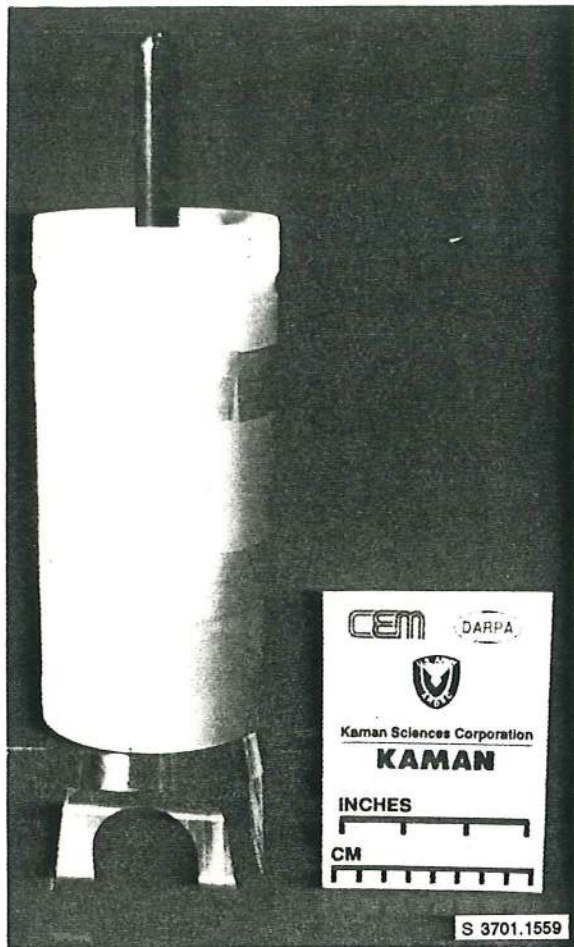
Figure 3. Kaman Sciences separating sabot and steel projectile launched by snubnose armature on shot #6 in 90-mm gun
