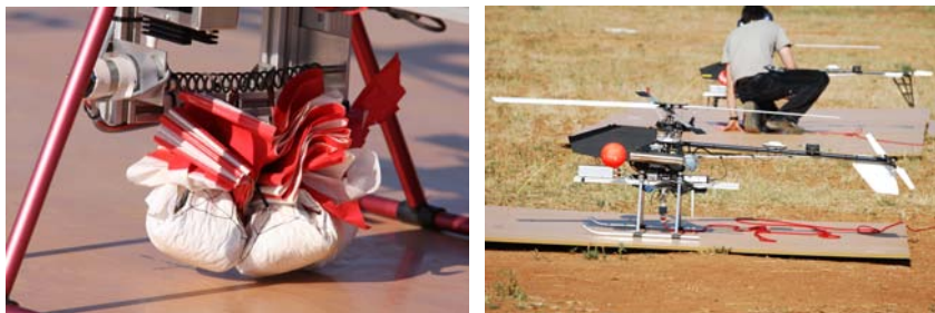
(a) Node Deployment Device (NDD) (b) TUB-H helicopter equipped with the LTD on the landing pad
