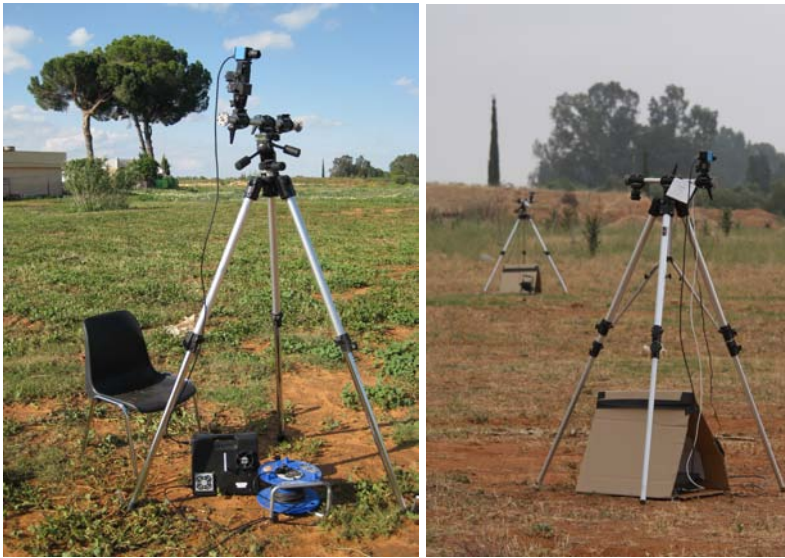
Fig. 8 Ground cameras used in the experimentation scenario. Each firewire camera was connected to a PC104 with a wireless link to the AWARE network.
